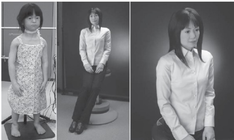
Fig. 3. The first android; Repliee R1 ( left : developed by Osaka University), and the latest android, Repliee Q2 ( right : developed by Osaka University and Kokoro Corporation)
